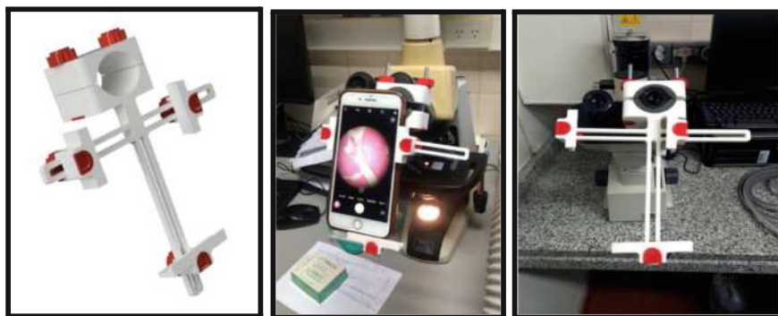
Fig. 3. Microscope eyepiece coupling prototype.
